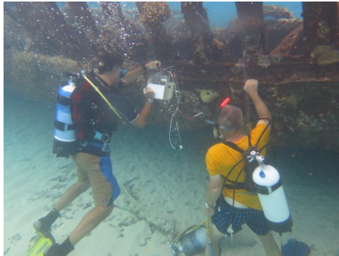
Figure 19. Corrosion survey being conducted on the shipwreck Phaeton , Cocos Island. D.Steinberg
